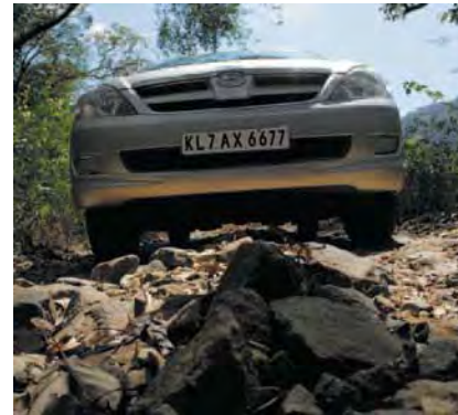
The shock absorbers in cars and trucks are heavily damped springs. The vehicle's vertical motion, after hitting a rock or a pothole, is a damped oscillation.
