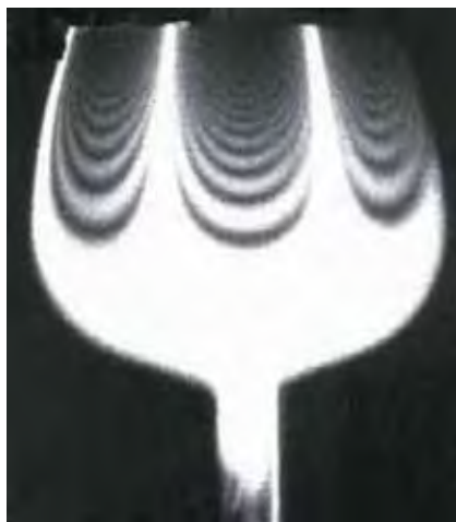
An optical technique called interferometry reveals the bell-like vibrations of a wine glass.
