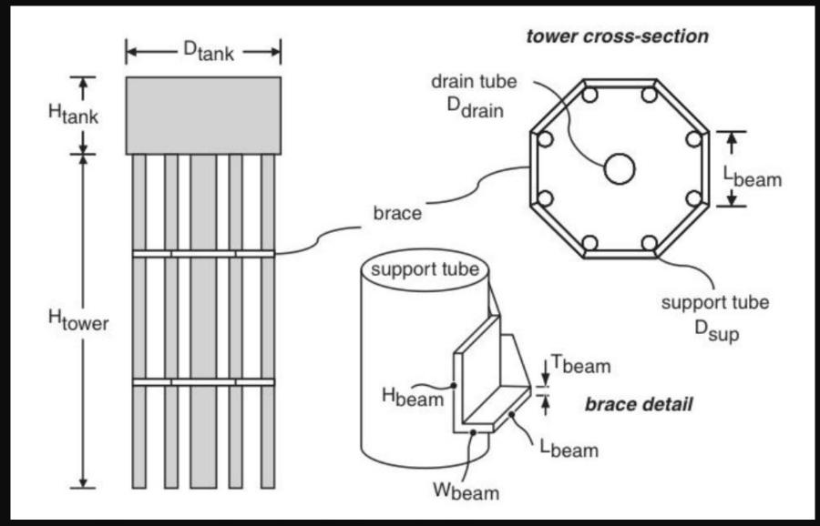
**Solution** The initial state in this problem is that we know the dimensions of the water tower. The goal state is to know the quantity of paint required to cover the tower. In developing the plan, we'll mainly use two heuristics: "working backwards" from the goal toward the initial state, and "divide and conquer" to break the tower into component parts.
