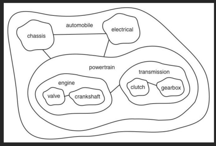
Using sub-systems leads to a better breakdown of the automobile
