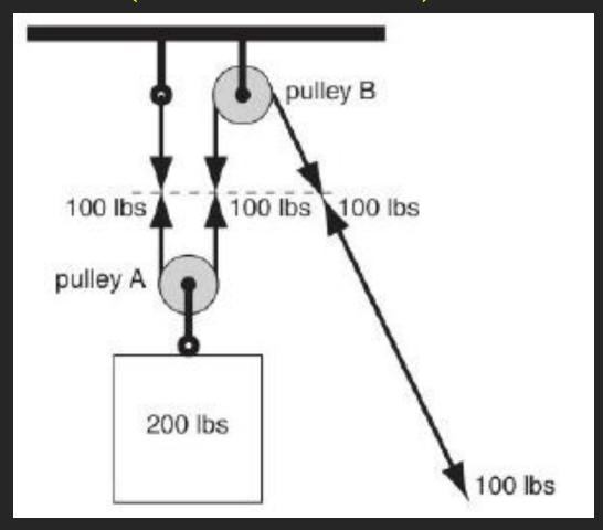
Because of the equal-and-opposite internal forces in the rope, each end of the segment around pulley A exerts an upward force of 100 lbs, for a total of 200 lbs.
